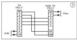
Installation of an additional telephone.
