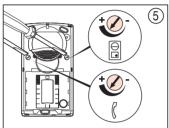
Adjust the volume of the telephone and Check the door opening. outdoor unit.
