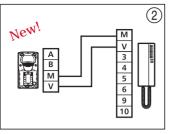
Automatic connection test. When the telephone is put back or the connection is wrong, the chimes are continuous.
