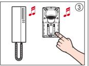
Press the button, the chimes ring at the outdoor unit and the telephone.
