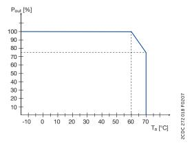
Characteristic curve of temperature at  $\mathbf{U}_{\text{out}}$
