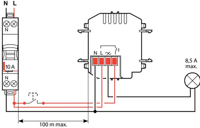
Pressing the auxiliary control allows the load to be switched on or off manually. If no action is performed on the control, the detector will cut off the related load at the end of the time delay or when the Daylight setpoint is reached.
